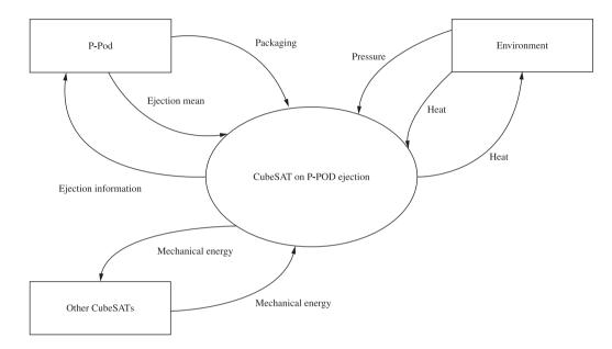
Figure 4. CubeSAT on P-POD ejection scenario - functional context diagram.
