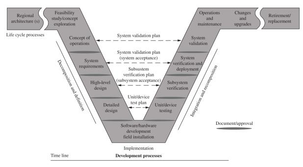
Figure 1. Model V diagram – Source: Kar and Bailey (1996).
