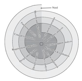
Figure 2. Spiral Diagram – Source: Kar and Bailey (1996).
