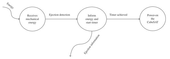
Figure 5. CubeSAT main functions in ejection scenario.
