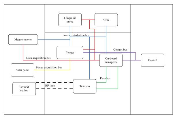
Figure 7. Architecture Interconnection Diagram – CubeSAT example.
