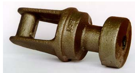
Figure 7 – Original casting part of a steel cable link.
