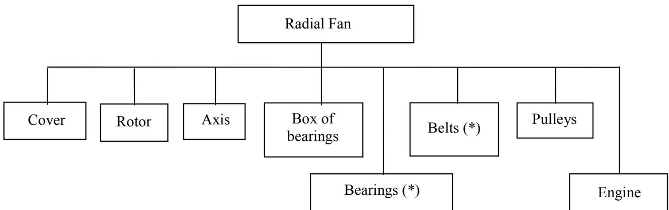
**Figure 6 – Structural tree of the radial fan.**
