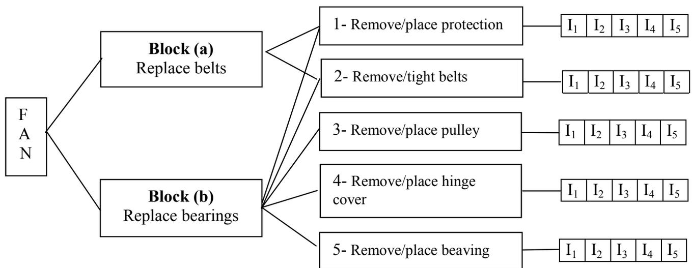
Figure 7 – Support tree with diagram of disassembly/assembly activities to “replace belts and bearings”.
